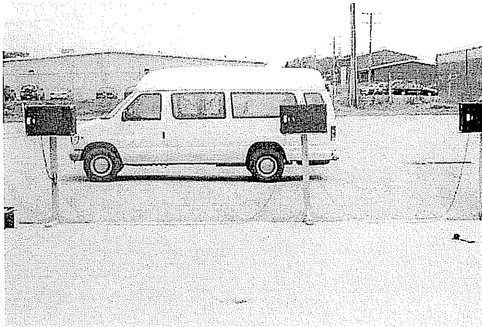
TEST VEHICLE SET-UP FOR 80 dB(A) INTERIOR NOISE TEST
